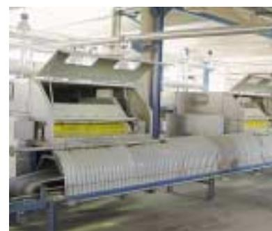
Sandvik Rotoform® units – discharge and conveying of sulphur pastilles
