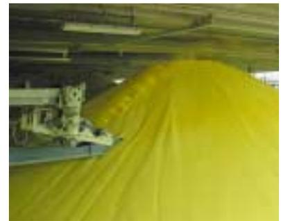
Econova's purpose-designed unit for depositing pastilles on the stockpile
