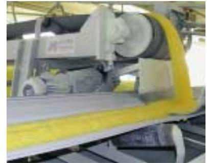
Rotoform® sulphur pastilles on the way to stockpile
