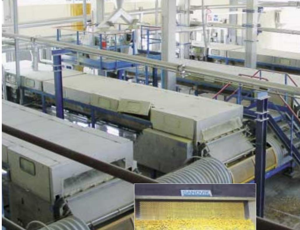
By 1992, the first complete turnkey installation had been put in operation at Melilli, near Syracuse. This system, consisting of sulphur pit, preconditioner, four steel belt coolers with Rotoformers<sup>®</sup> and the cooling water tower, was designed for 24 hour a day operation, 365 days a year, and has been processing up to 300 tons a day ever since.
