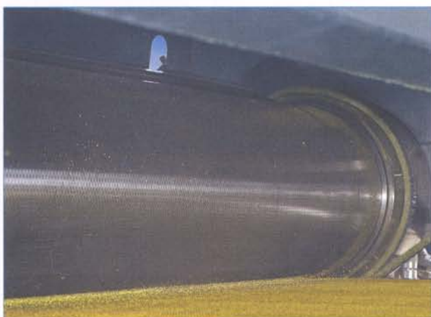
Figure 4. The larger diameter, 'dropformer' perforated shell, which deposits the sulfur droplets.
